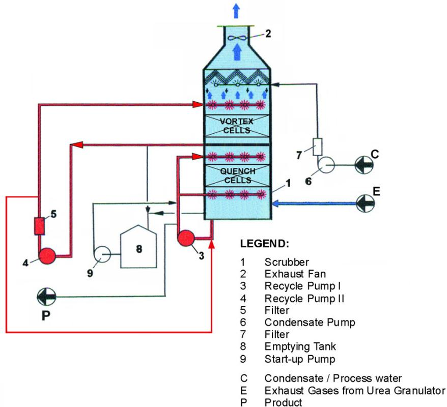
Fig. 5. Cleaning the air coming from urea granulators in the CLEANING UNIT by PROZAP (Poland)
