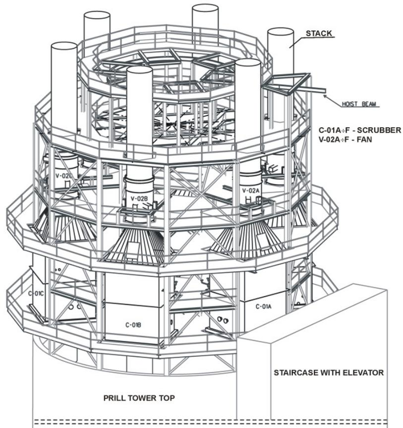
Fig.8. Placing scrubbers on top of a prilling tower
