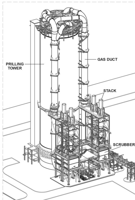
Fig.10. Placing PROZAP's CLEANING UNIT scrubbers on the ground level
